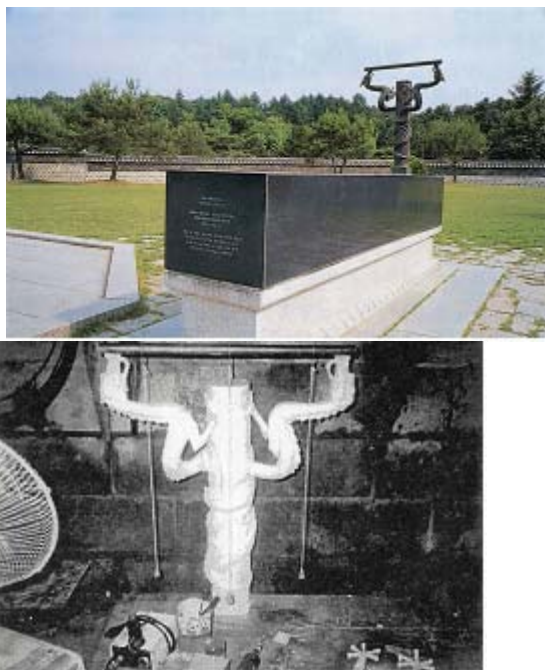
Figure 11. A recent reproduction by Nha [7] at 10% scale of the recorded size of King Sejong's High Gnomon is shown (left). The Measuring Scale is 260 cm long and the height of the rod on the gnomon is 70 cm. (1 Yuan foot = 24.5 cm and 1 Joseon foot = 20.7 cm)
