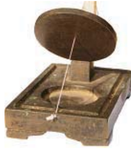
Figure 12. A Korean copy of the Xuanzheng-yi 懸正儀, Correcting-Instrument with Pendulum, by Guo Shoujing. Its Korean name is presumed to be Hyonju Ilgui 懸珠日晷.
